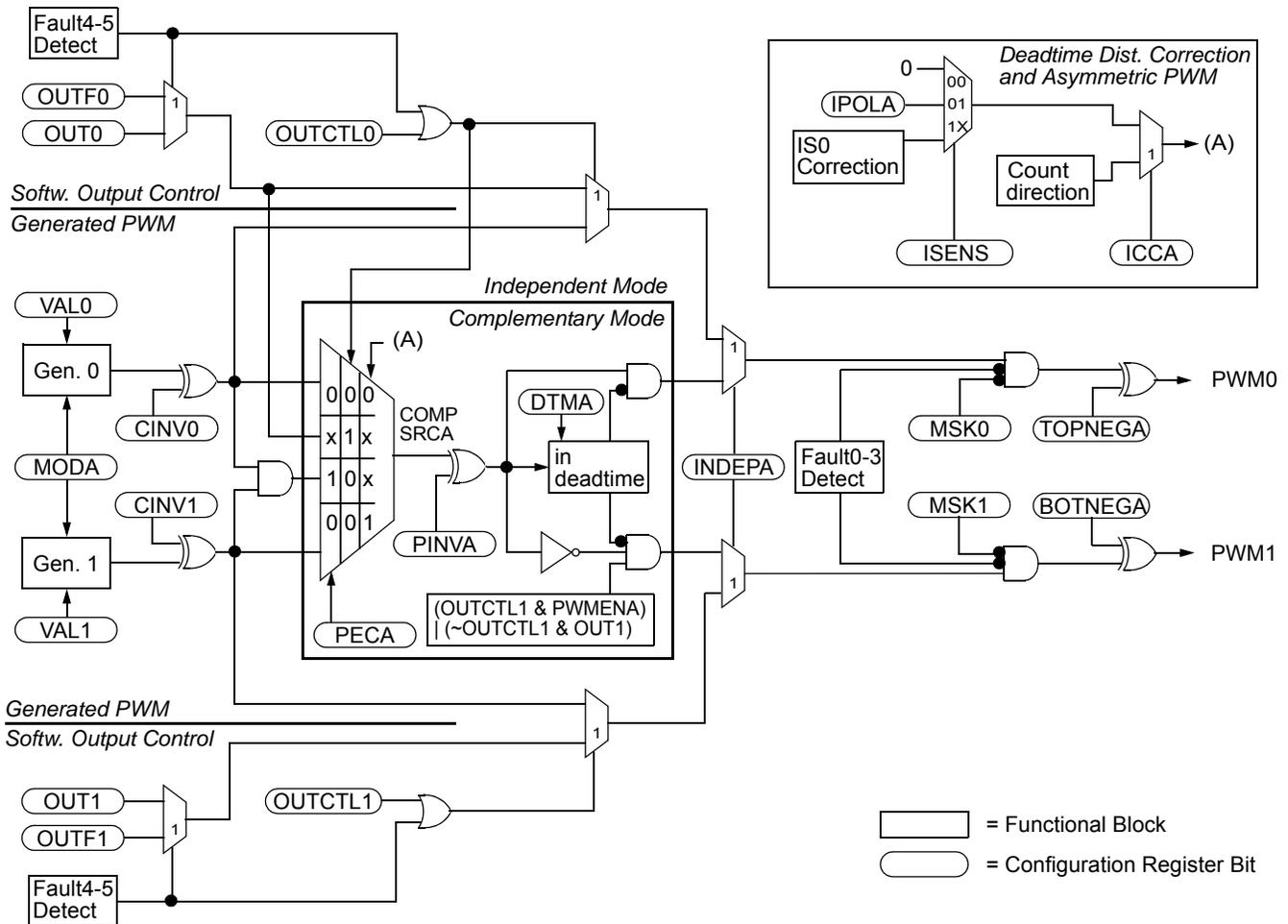
Figure 15-41. Detail of PWM0 and PWM1 Signal Paths
