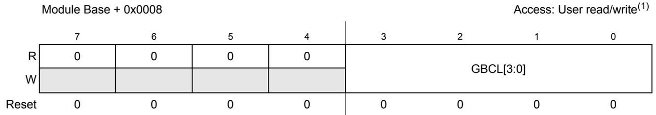
Figure 18-11. GDU Boost Current Limit Register (GDUBCL)
