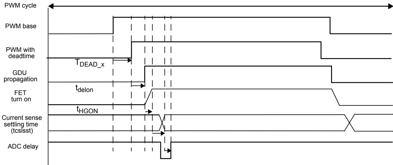
The PWM deadtime ( $T_{DEAD\_X}$ ) is an integral number of bus clock cycles, configured by the PMF deadtime registers.
