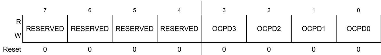
Figure 11-20. Output Compare Pin Disconnect Register (OCPD)
