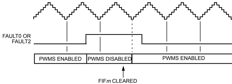
Figure 15-85. Manual Fault Recovery (Faults 0 and 2) — QSMP = 01, 10, or 11
