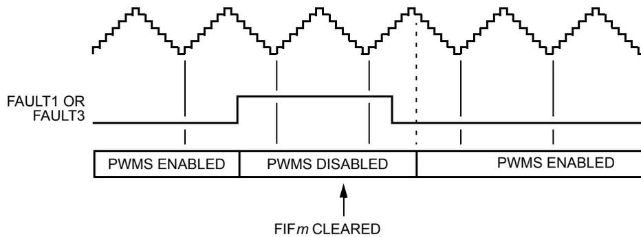
Figure 15-86. Manual Fault Recovery (Faults 1 and 3-5)
