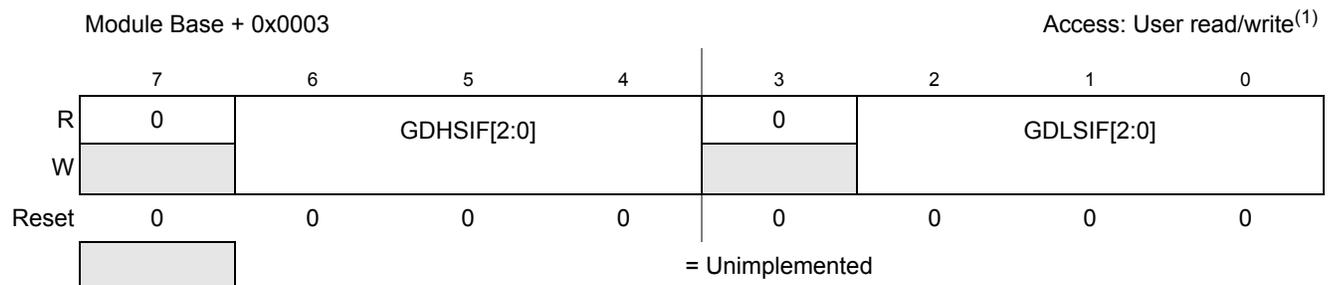
**Figure 18-6. GDU Desaturation Error Flag Register (GDUDSE)**
