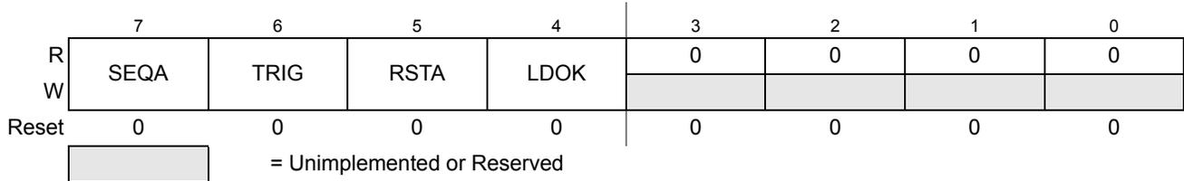
Figure 9-9. ADC Conversion Flow Control Register (ADCFLWCTL)
