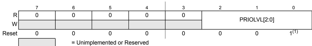
Figure 4-5. Interrupt Request Configuration Data Register 0 (INT\_CFDATA0)
