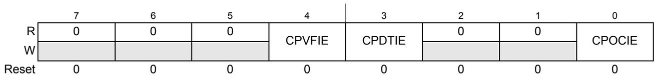
Figure 21-8. CAN Physical Layer Interrupt Enable Register (CPIE)
