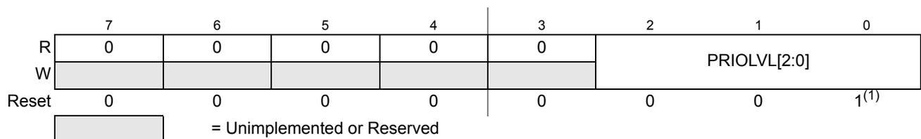
Figure 4-6. Interrupt Request Configuration Data Register 1 (INT\_CFDATA1)
