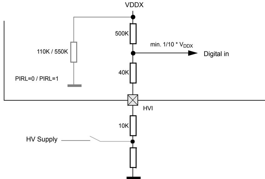
**Figure 2-38. Digital Input Read with Pullup Enabled**
