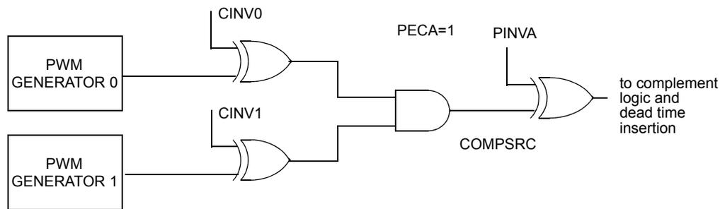
Figure 15-63. Logic AND Function with Signal Inversions
