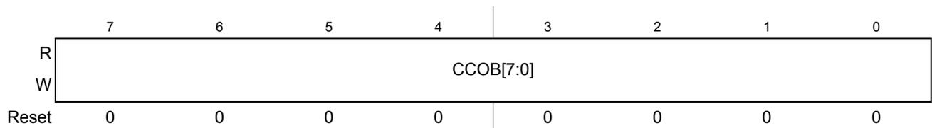
Figure 20-23. Flash Common Command Object 2 Low Register (FCCOB2LO)
