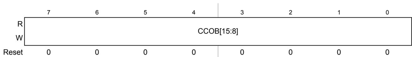
Figure 20-26. Flash Common Command Object 4 High Register (FCCOB4HI)
