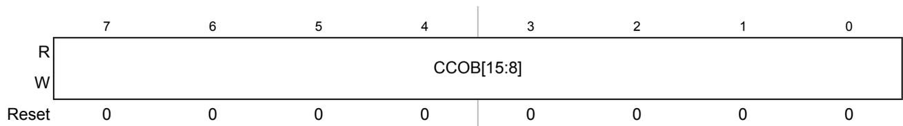
Figure 20-24. Flash Common Command Object 3 High Register (FCCOB3HI)
