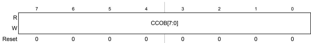
Figure 20-25. Flash Common Command Object 3 Low Register (FCCOB3LO)
