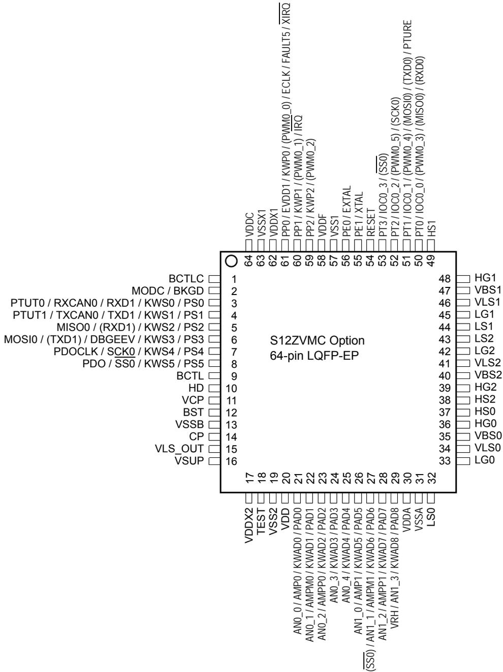
Figure 1-5. S12ZVMC Option 64-pin LQFP pin out
