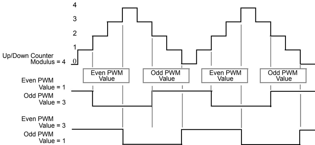
Figure 15-62. Asymmetric Waveform - Phase Shift PWM Output
