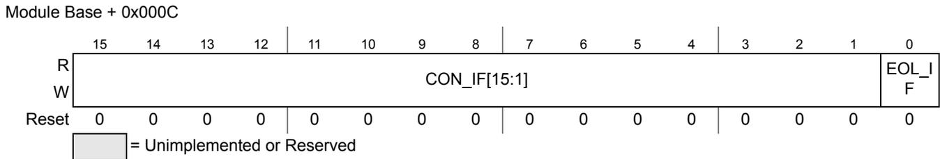
Figure 9-15. ADC Conversion Interrupt Flag Register (ADCCONIF)
