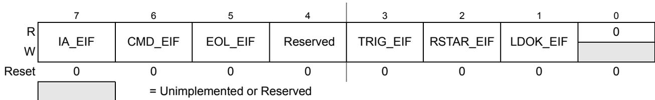
**Figure 9-12. ADC Error Interrupt Flag Register (ADCEIF)**
