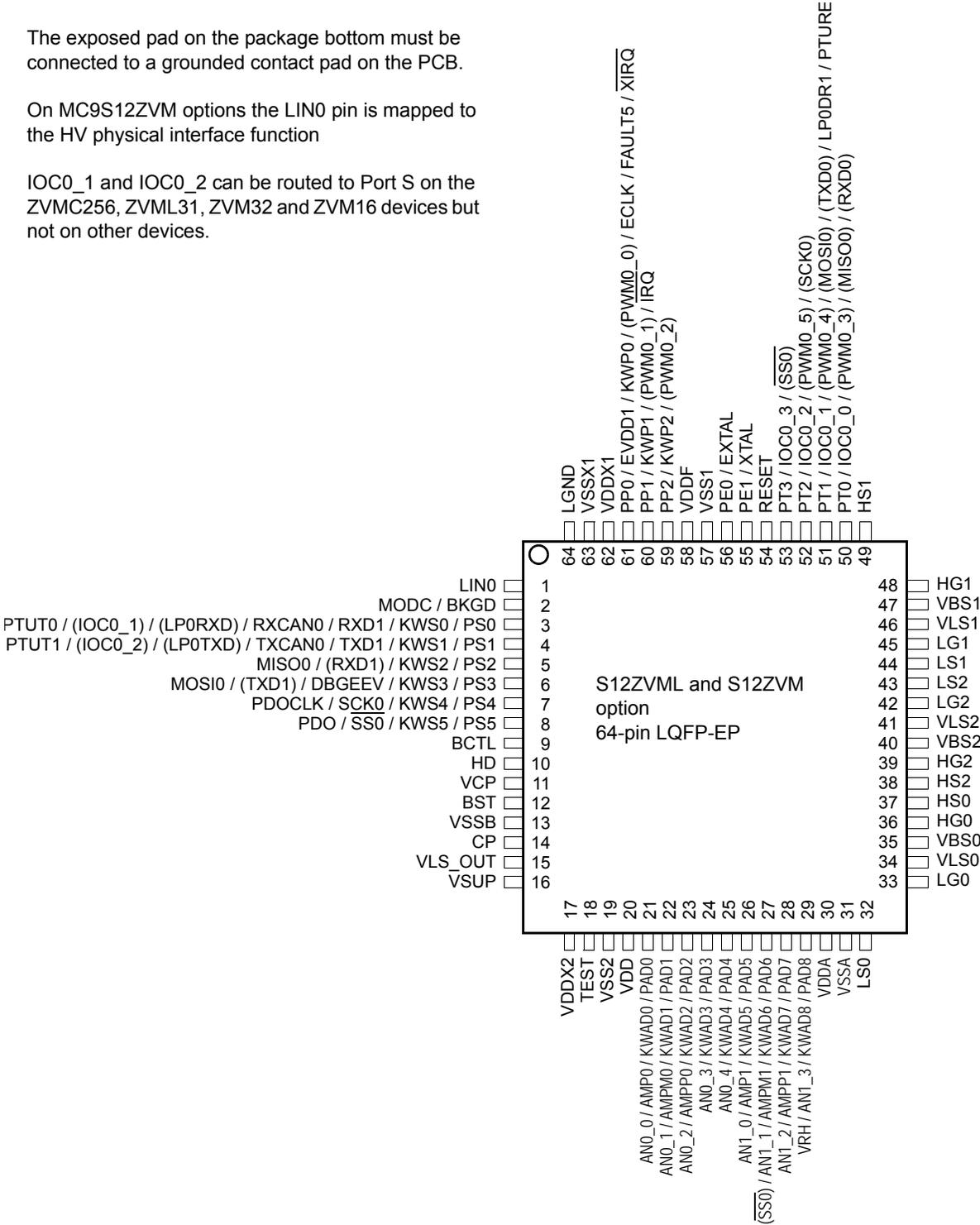
Figure 1-4. S12ZVM and S12ZVM L option 64-pin LQFP pin out
