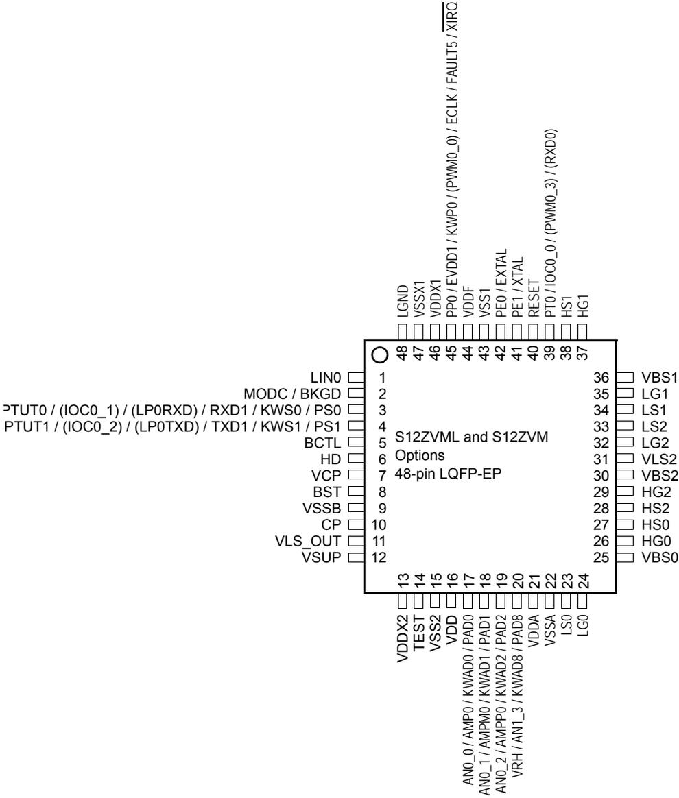
Figure 1-6. S12ZVM, S12ZVML Option 48-pin LQFP
