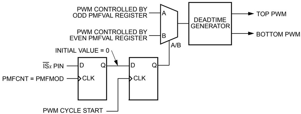
Figure 15-59. Internal Correction Logic when ISENS = 11
