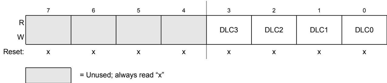
**Figure 13-35. Data Length Register (DLR) — Extended Identifier Mapping**
