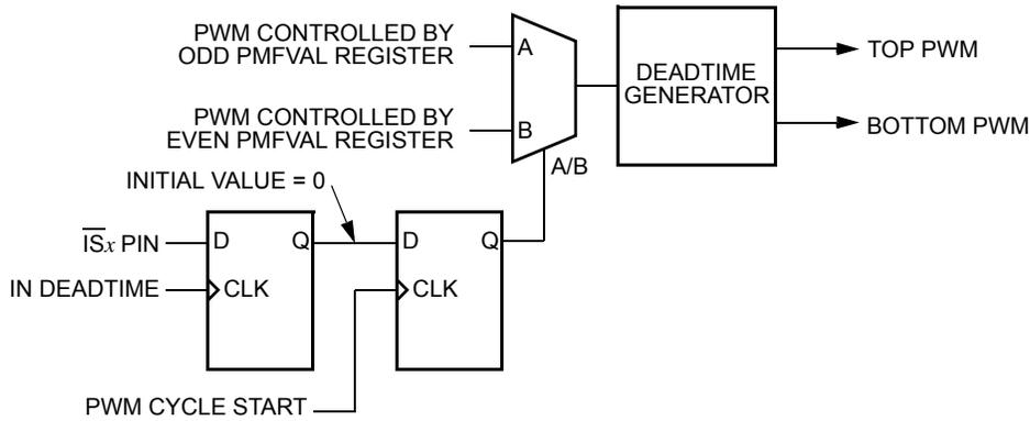
Figure 15-58. Internal Correction Logic when ISENS = 10
