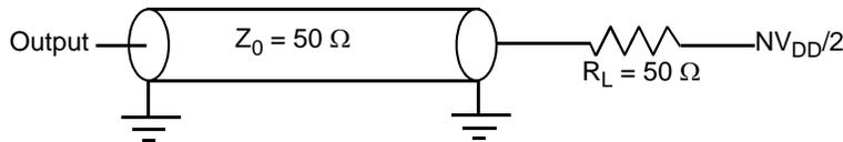
**Figure 40. AC Test Load for the JTAG Interface**
