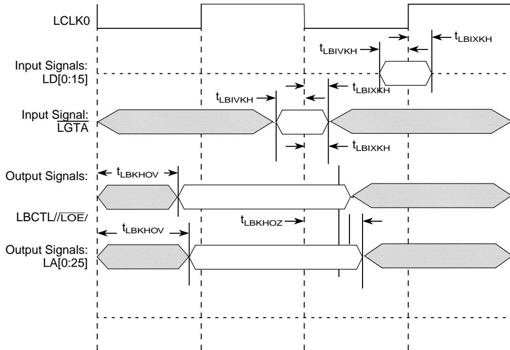
Figure 31. Local Bus Signals, Non-Special Signals Only
