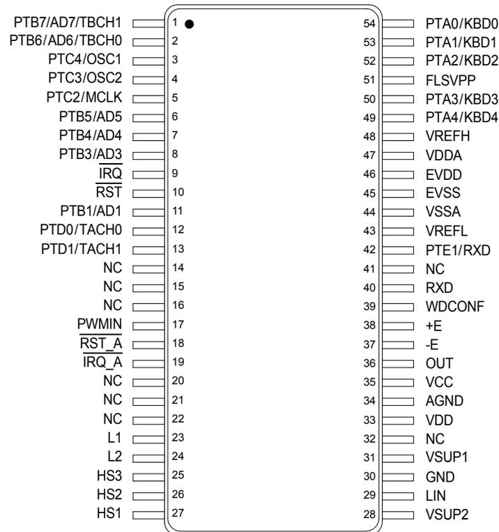
Figure 3. Pin Connections
