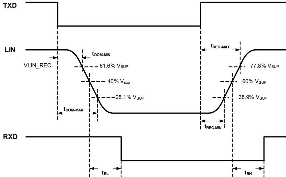
Figure 7. LIN Timing Measurements for Slow Slew Rate
