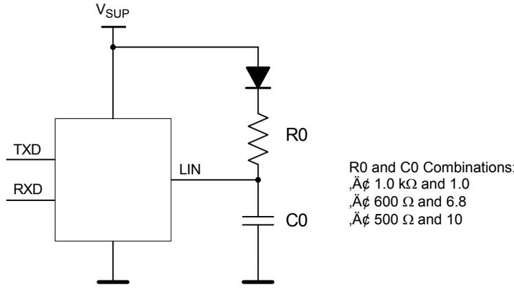
Figure 5. Test Circuit for LIN Timing Measurements
