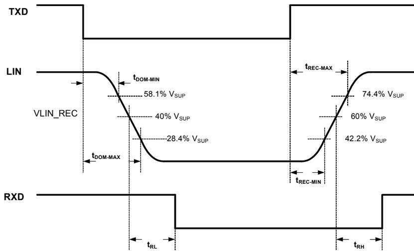
Figure 6. LIN Timing Measurements for Normal Slew Rate
