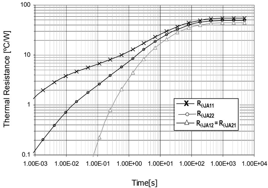
Figure 24. Transient Thermal Resistance R<sub>θJA</sub> (1.0 W Step Response)
