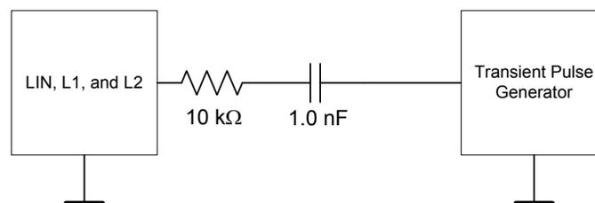
**Note** Waveform in accordance with ISO7637 Part 1, Test Pulses 1, 2, 3a, and 3b.
