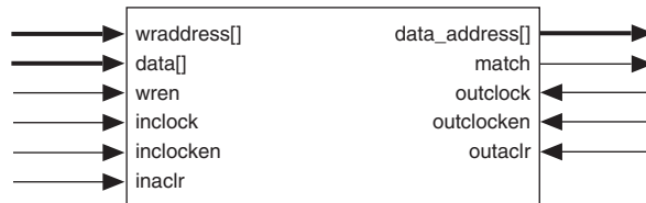
Figure 23. APEX 20KC CAM Block Diagram
