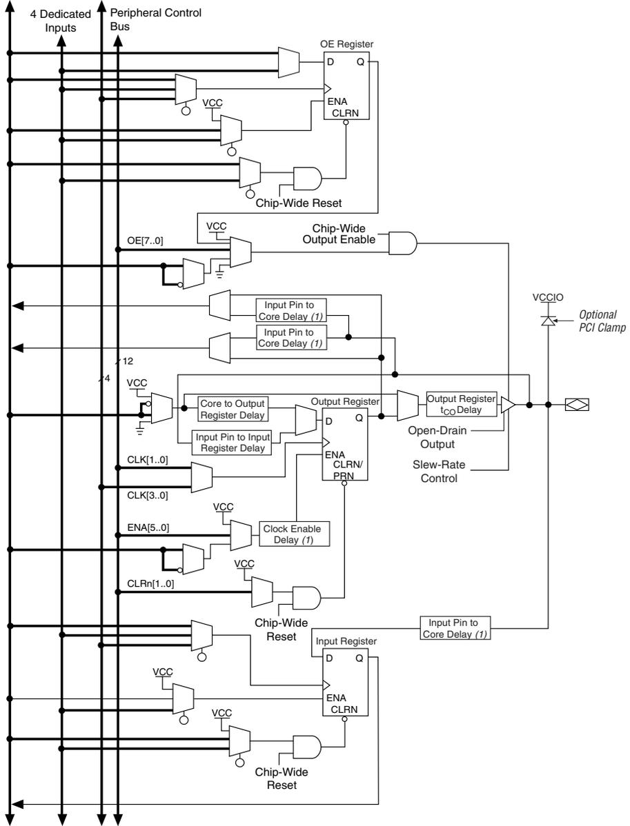
Figure 27 shows how a column IOE connects to the interconnect.
