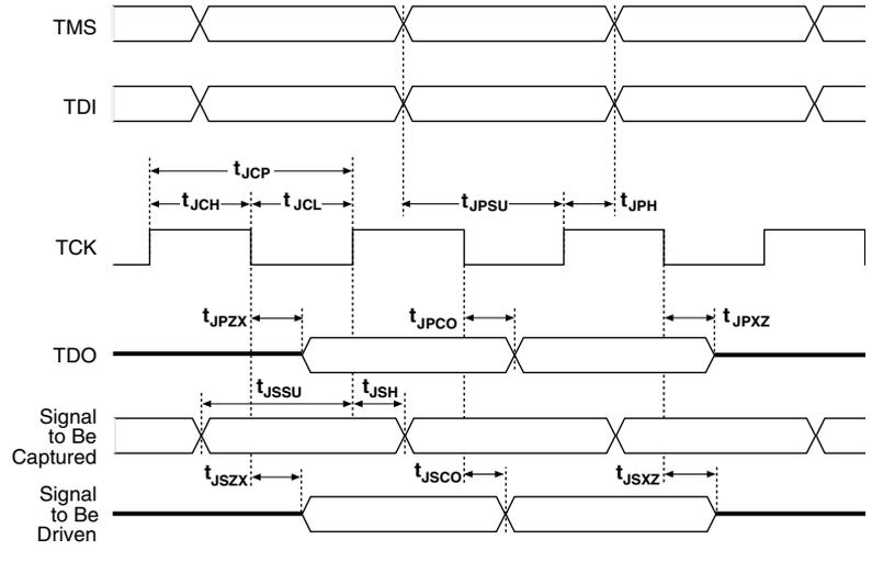
Table 16 shows the JTAG timing parameters and values for APEX 20KC devices.
