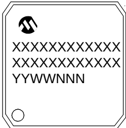
100-Lead TQFP (14x14x1 mm)
