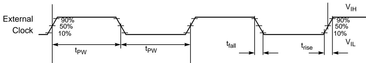
Note: The midpoint is  $V_{IL} + (V_{IH} - V_{IL})/2$ .
