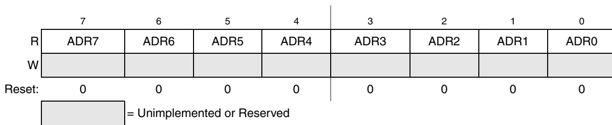
Figure 9-7. Data Result Low Register (ADCRL)
