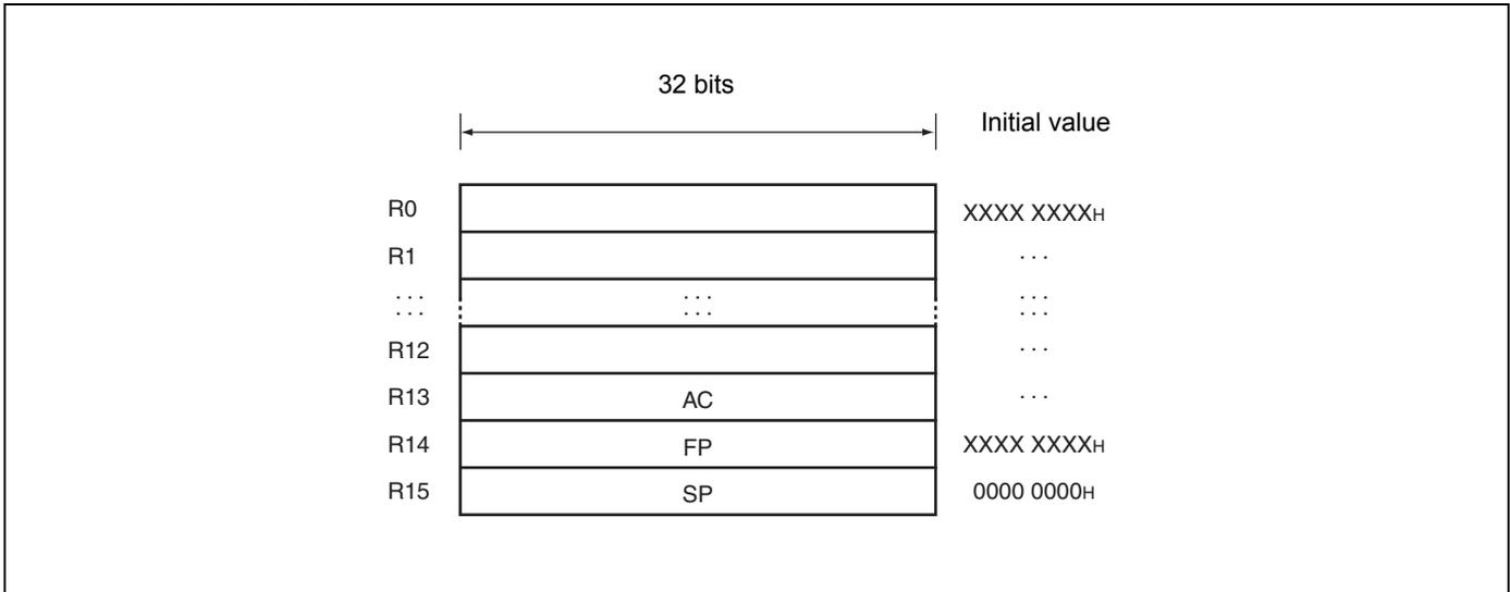
Registers R0 to R15 are general-purpose registers. These registers can be used as accumulators for computation operations and as pointers for memory access.
