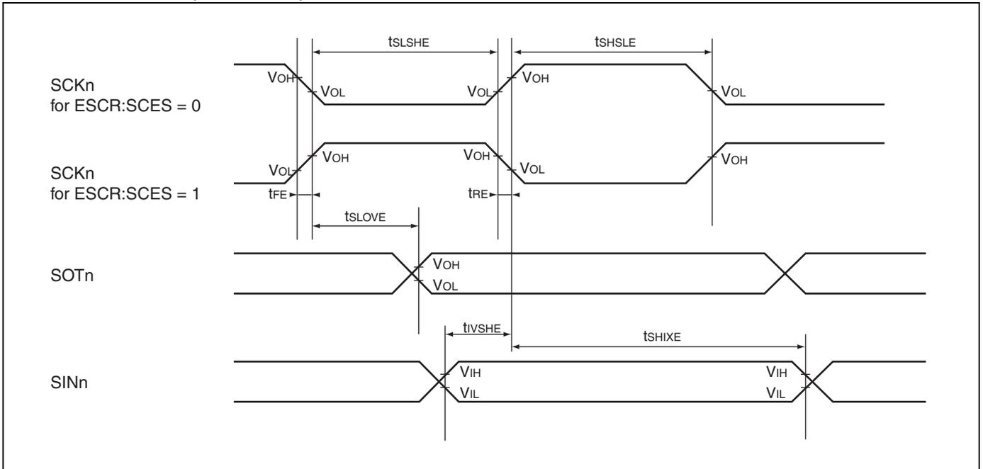
**Synchronous/Asynchronous read access**
