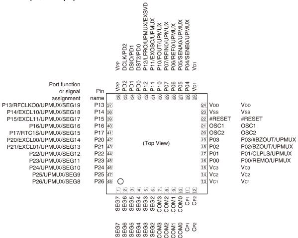
**Note**: The model in this package cannot be placed into super economy mode, as it does not have the V<sub>D2</sub>, C<sub>V1</sub>, and C<sub>V2</sub> pins.
