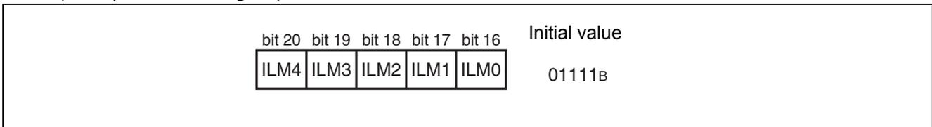
This register stores interrupt level mask values, and the values stored in ILM4 to ILM0 are used for level masking.
