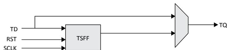
**Figure 2.21. Tristate Register Block on Top Side**
