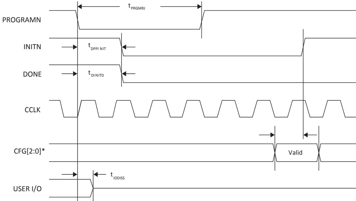
\*The CFG pins are normally static (hardwired).
