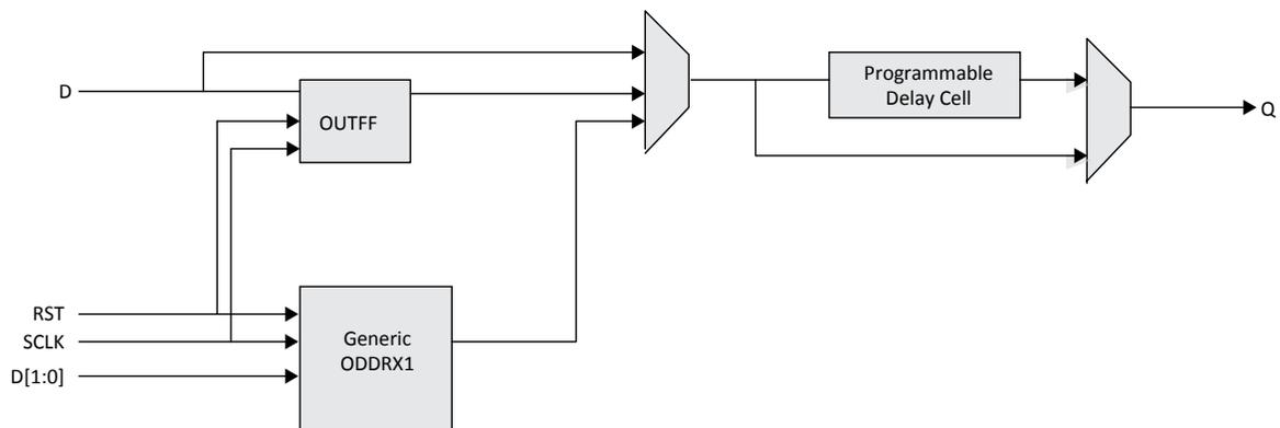
**Figure 2.19. Output Register Block on Top Side**
