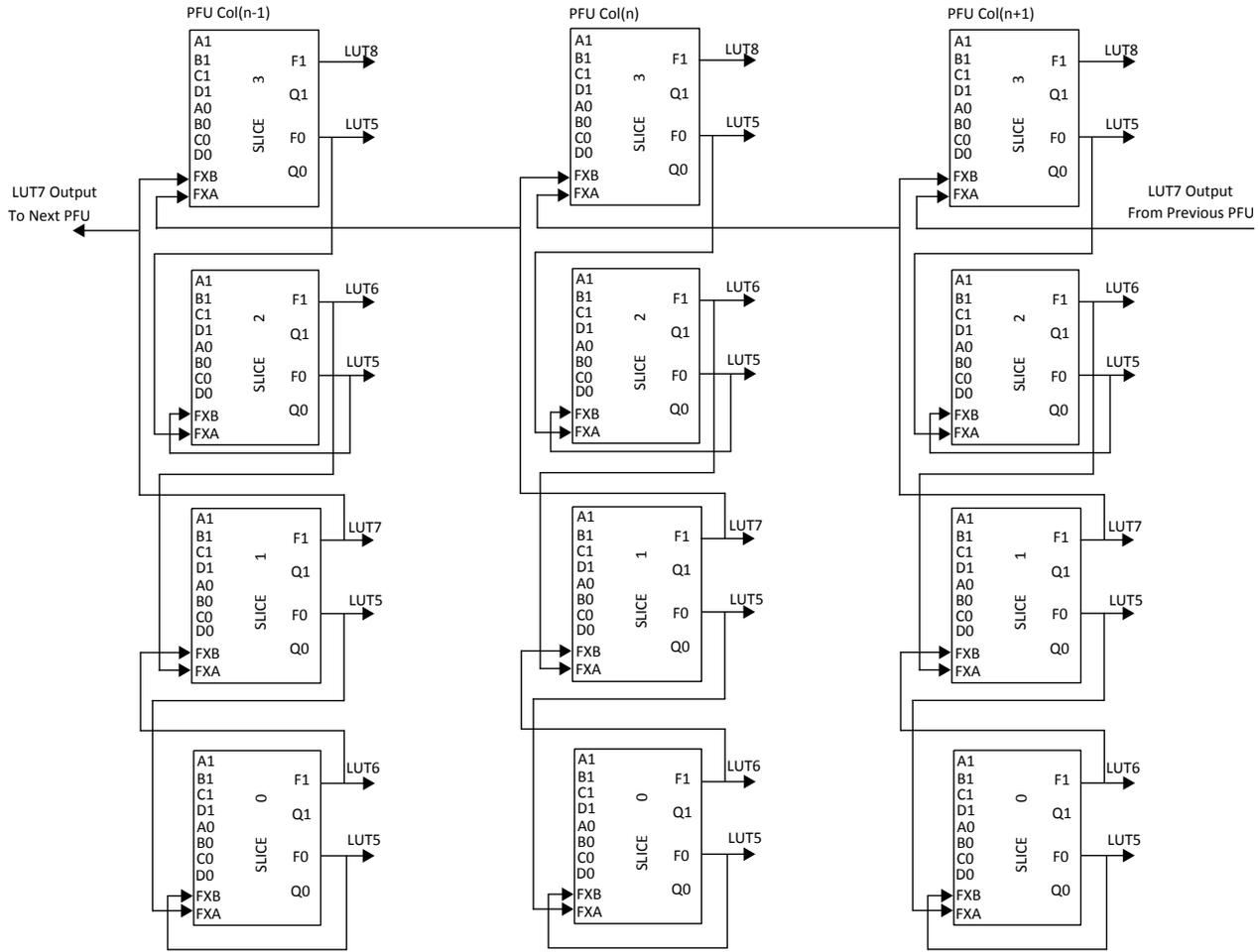
Figure 2.4. Connectivity Supporting LUT5, LUT6, LUT7, and LUT8
