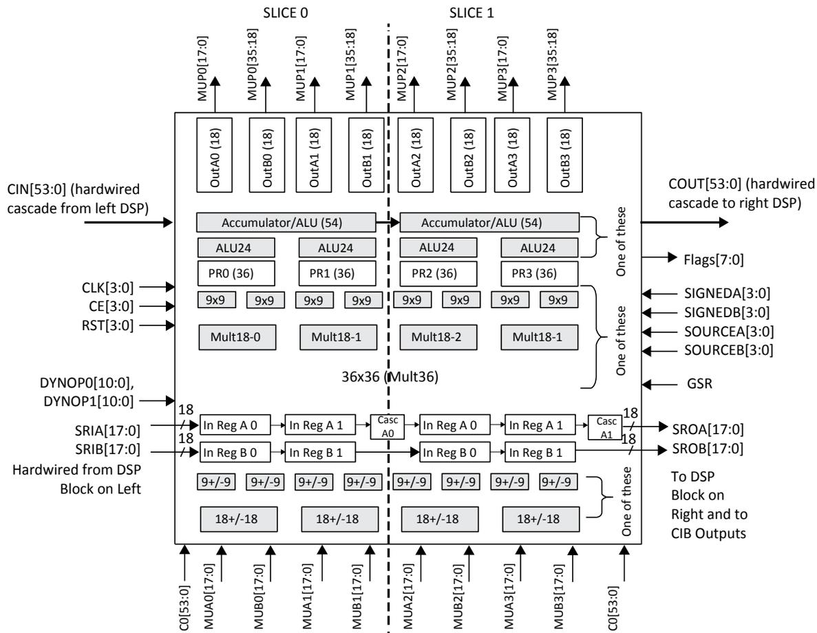
**Figure 2.14. Simplified sysDSP Slice Block Diagram**
