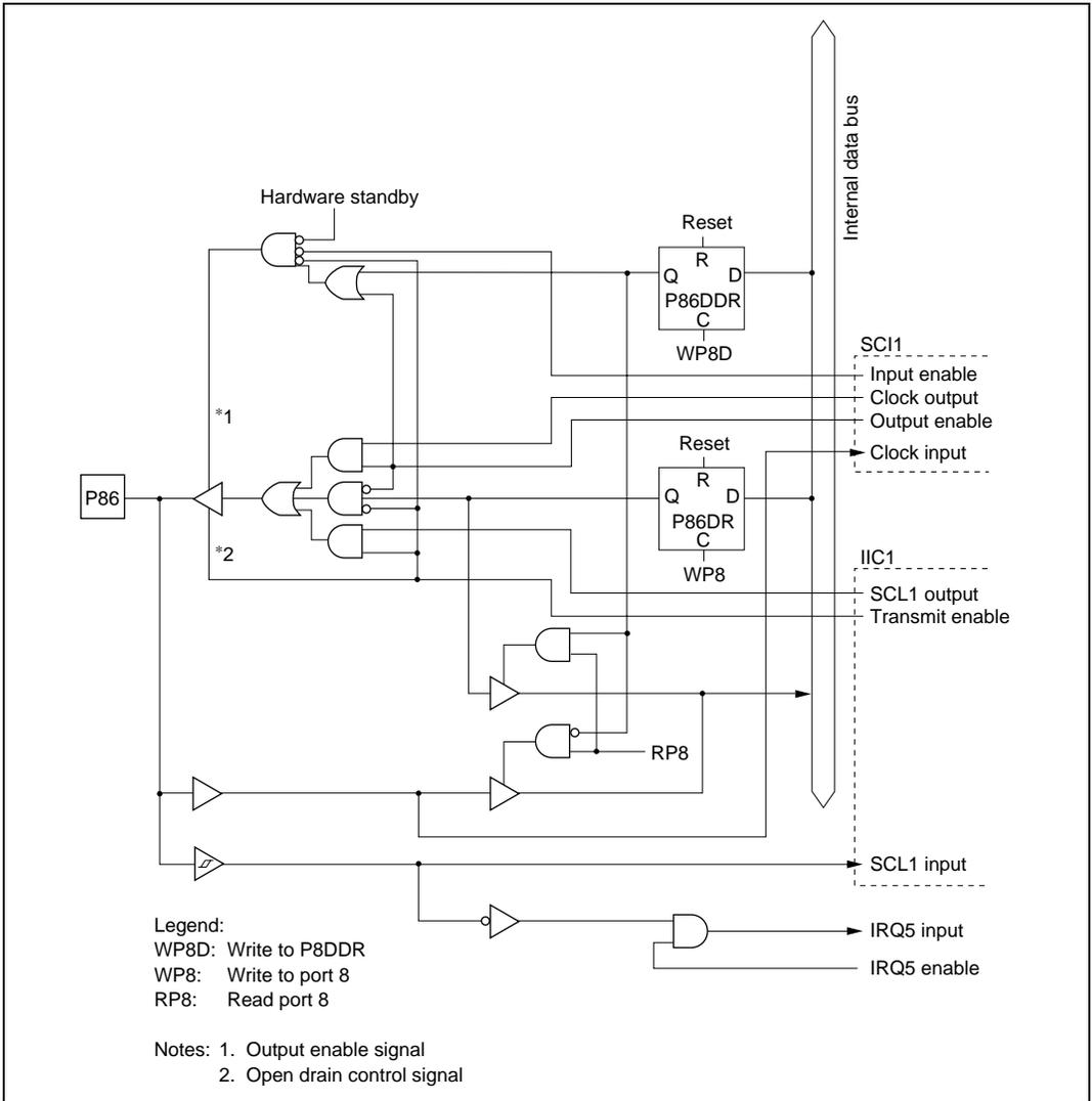
Figure C.28 Port 8 Block Diagram (Pin P86)
