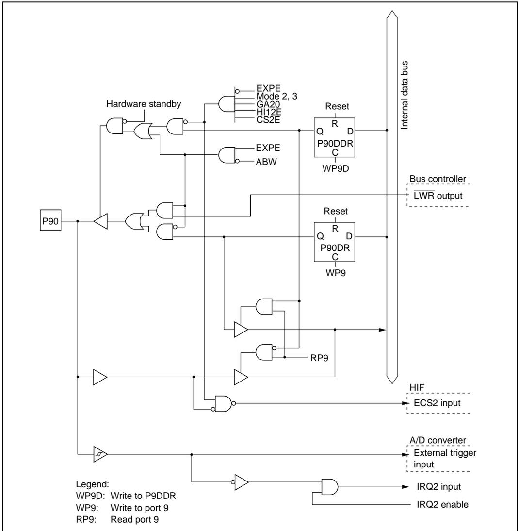
**Figure C.29 Port 9 Block Diagram (Pin P90)**
