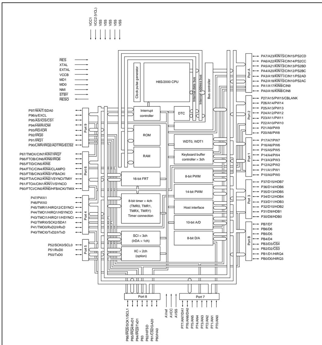
Figure 1.1 (a) Internal Block Diagram of H8S/2148 Group
