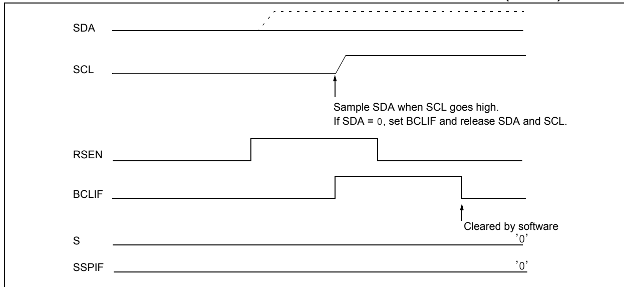
FIGURE 30-36: BUS COLLISION DURING A REPEATED START CONDITION (CASE 1)
