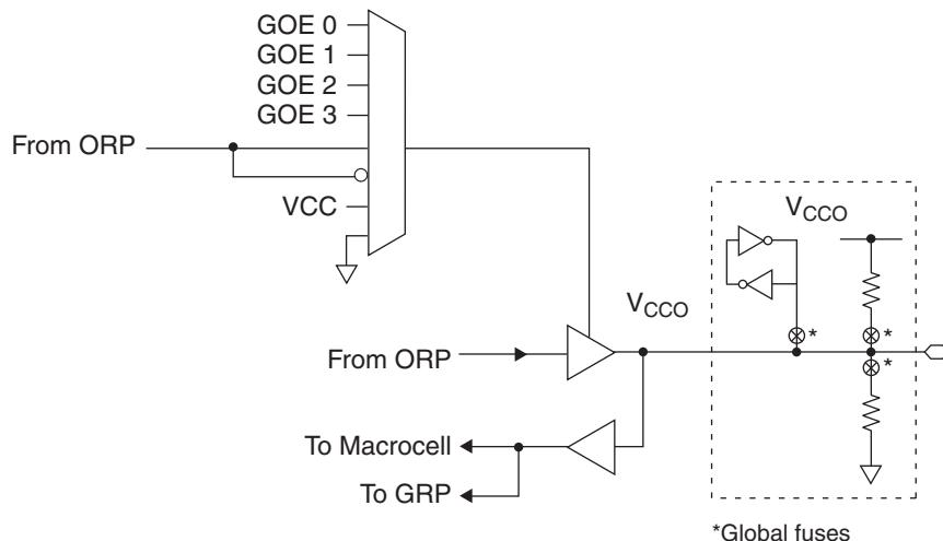
Each output supports a variety of output standards dependent on the  $V_{CCO}$  supplied to its I/O bank. Outputs can also be configured for open drain operation. Each input can be programmed to support a variety of standards, independent of the  $V_{CCO}$  supplied to its I/O bank. The I/O standards supported are:
