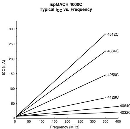
Note: The devices are configured with maximum number of 16-bit counters, typical current at 1.8V, 25°C.
