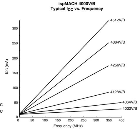
Note: The devices are configured with maximum number of 16-bit counters, typical current at 3.3V, 2.5V, 25°C.
