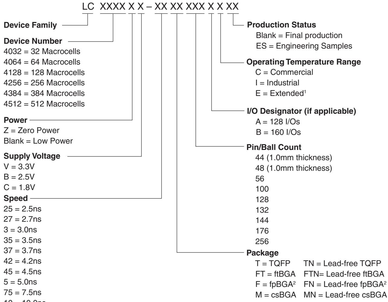
1. For automotive AEC-Q100 compliant devices, refer to the LA-ispmach 4000V/Z Automotive Family Data Sheet (DS1017).
