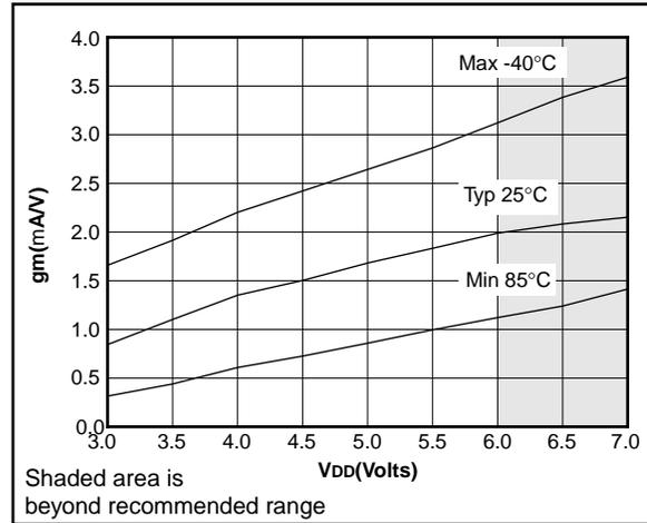
**FIGURE 21-20: TRANSCONDUCTANCE(g<sub>m</sub>) OF LP OSCILLATOR vs. V<sub>DD</sub>**
