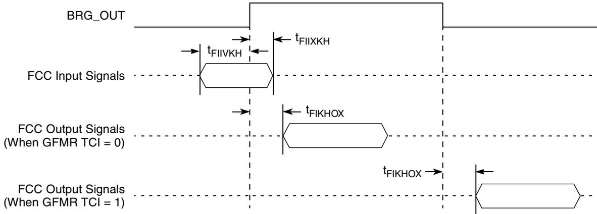
Figure 24. FCC Internal AC Timing Clock Diagram
