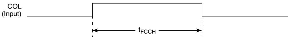
Figure 26. Ethernet Collision AC Timing Diagram (FCC)
