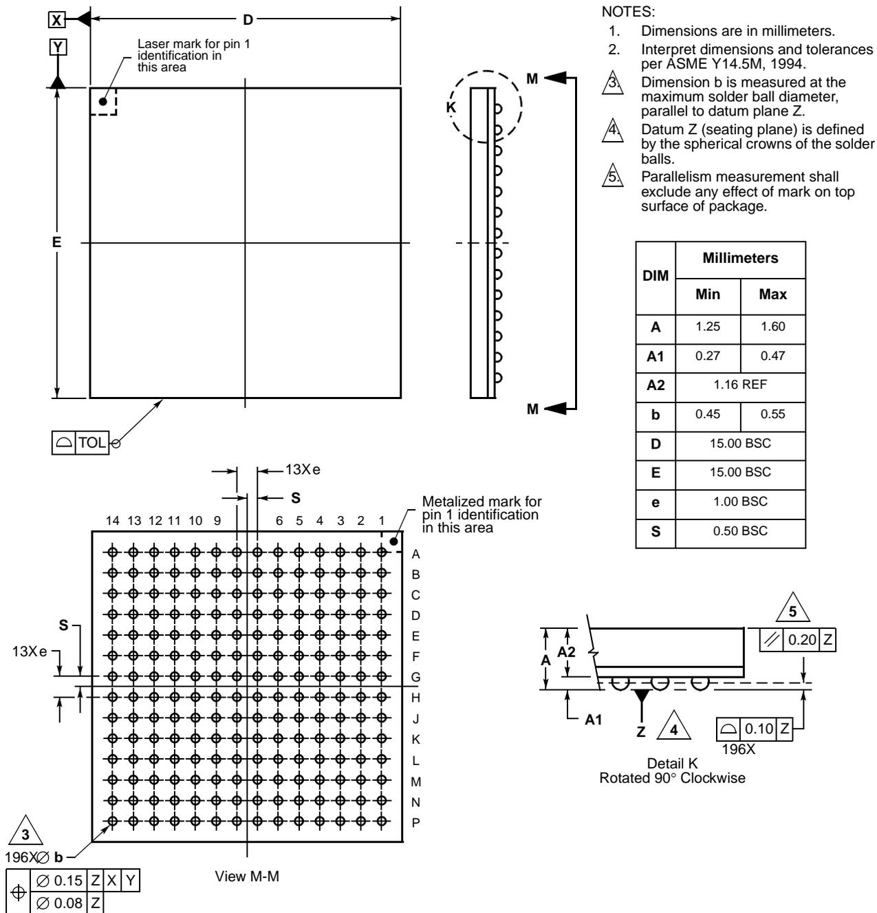
Figure 4. 196 MAPBGA Package Dimensions (Case No. 1128A-01)
