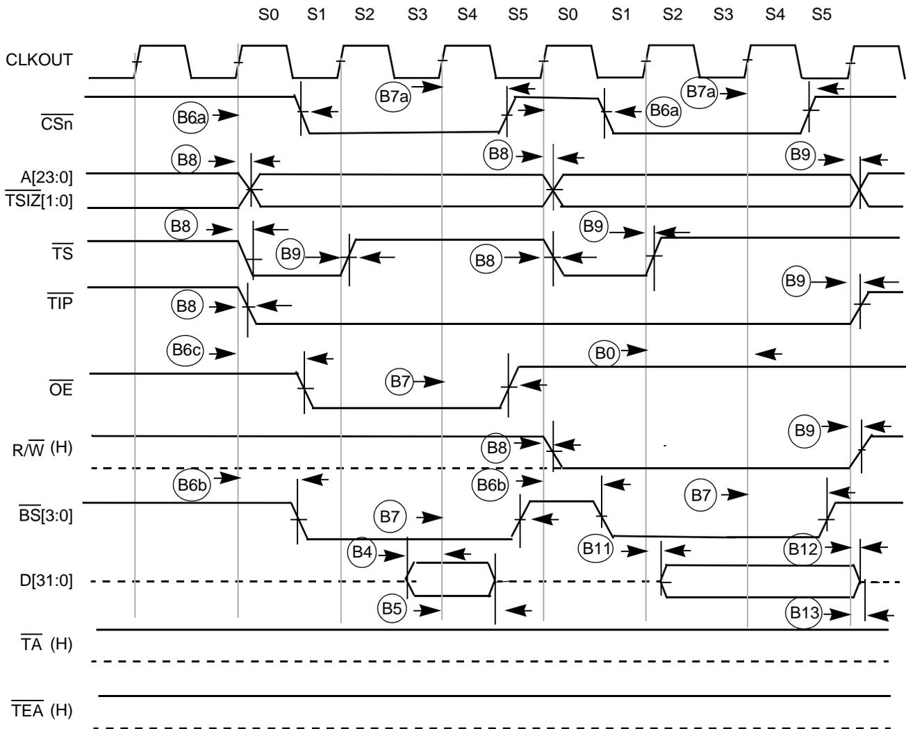
Figure 8. Read/Write (Internally Terminated) SRAM Bus Timing
