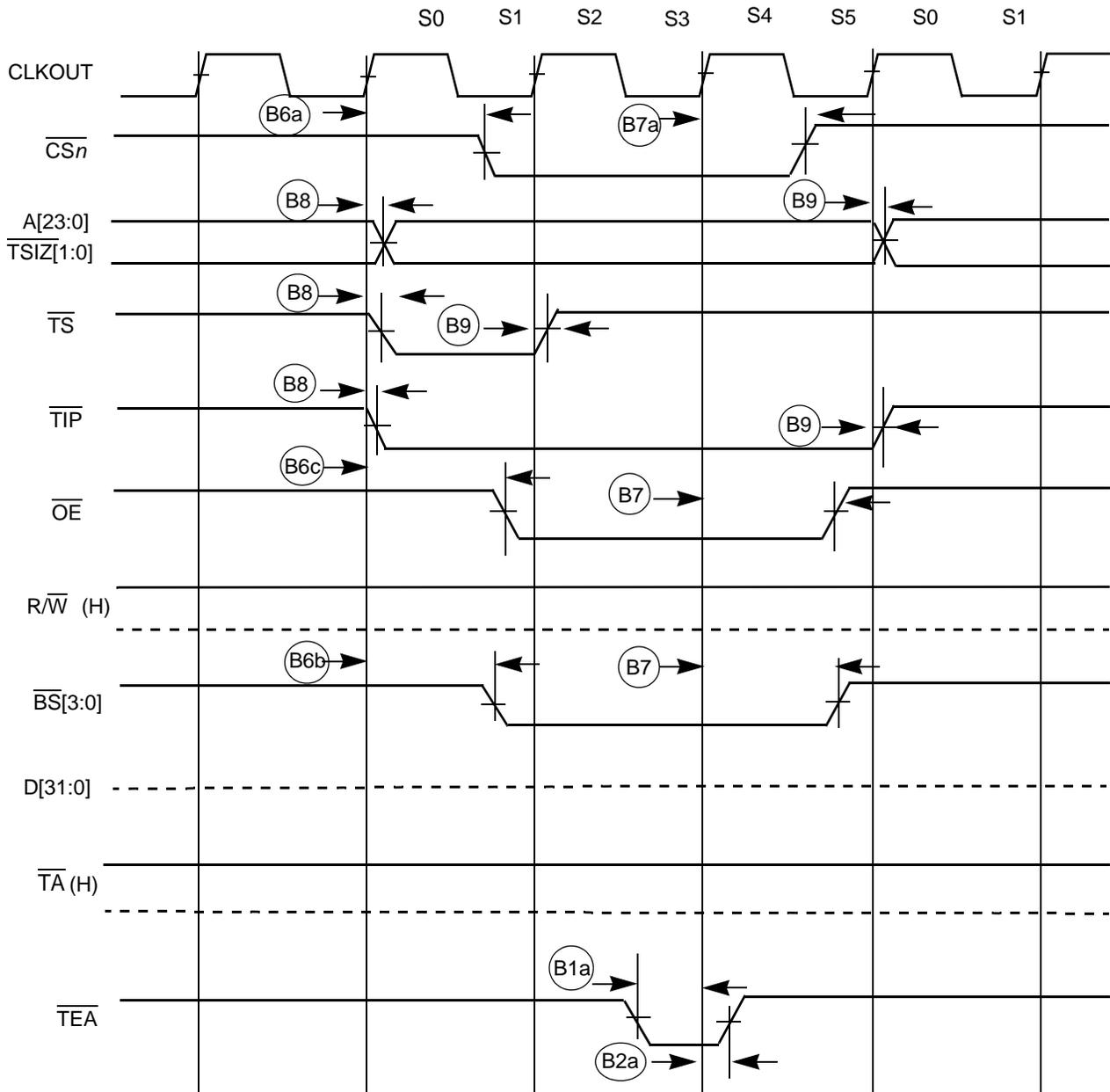
Figure 10. SRAM Read Bus Cycle Terminated by  $\overline{TEA}$
