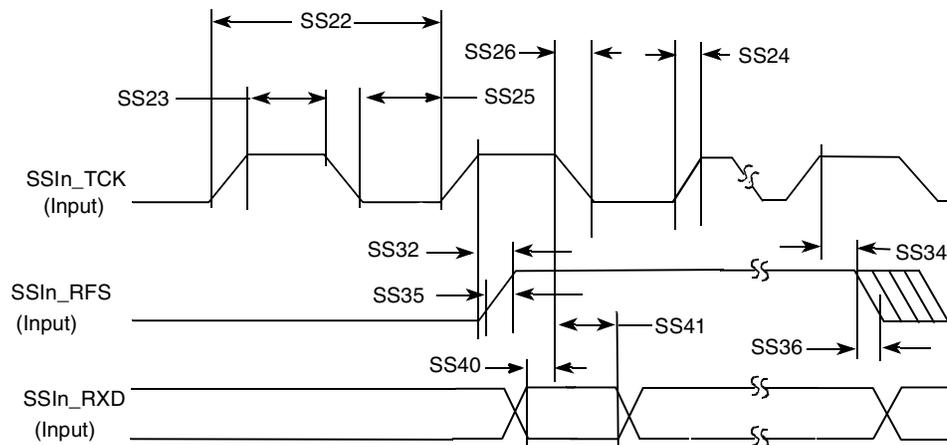
**Figure 20. SSI Receiver with External Clock Timing Diagram**
