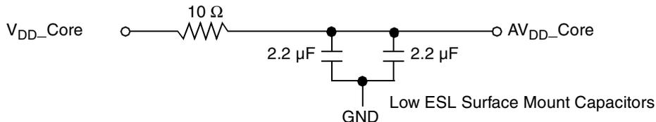
Figure 49. MPC8610 PLL Power Supply Filter Circuit (for Core)
