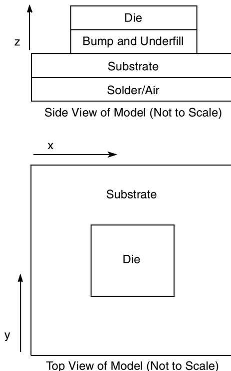
Figure 57. MPC8610 Thermal Model
