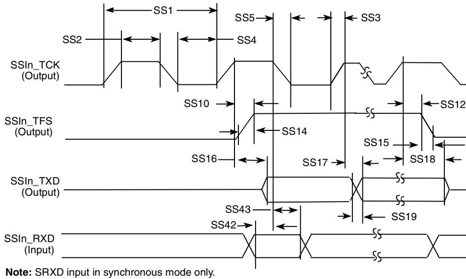
**Figure 17. SSI Transmitter with Internal Clock Timing Diagram**
