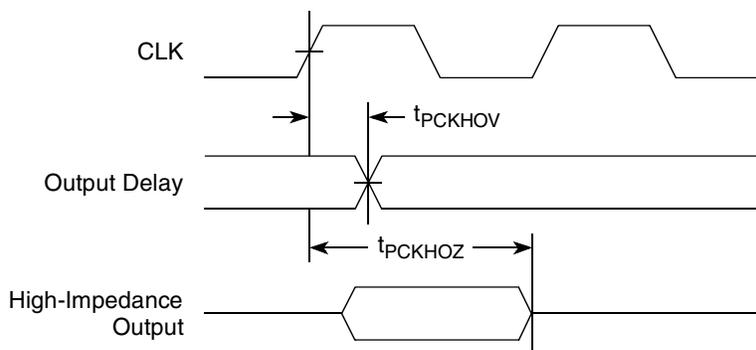
Figure 28. PCI Output AC Timing Measurement Condition
