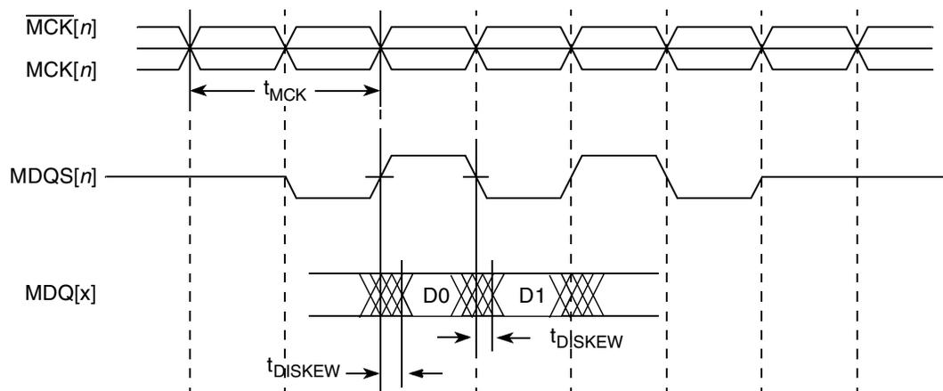
**Figure 4. DDR Input Timing Diagram for  $t_{DISKEW}$**
