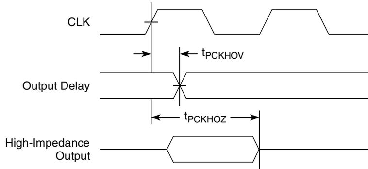
Figure 28. PCI Output AC Timing Measurement Condition
