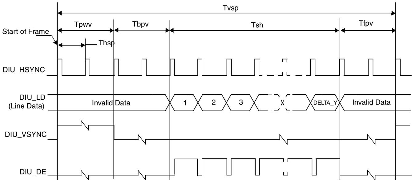
Figure 13. TFT DIU/LCD Interface Timing Diagram—Vertical Sync Pulse
