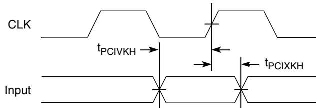
**Figure 27. PCI Input AC Timing Measurement Conditions**
