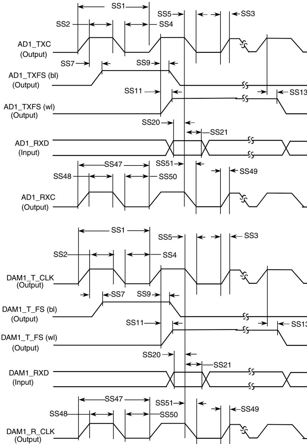
Figure 93. SSI Receiver with Internal Clock Timing Diagram
