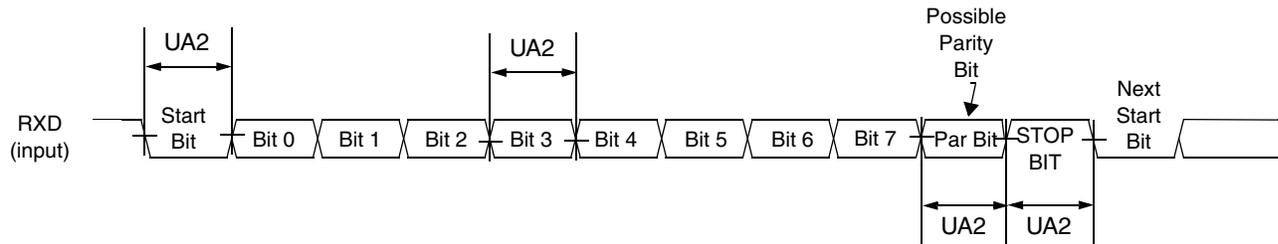
**Figure 97. UART RS-232 Serial Mode Receive Timing Diagram**
