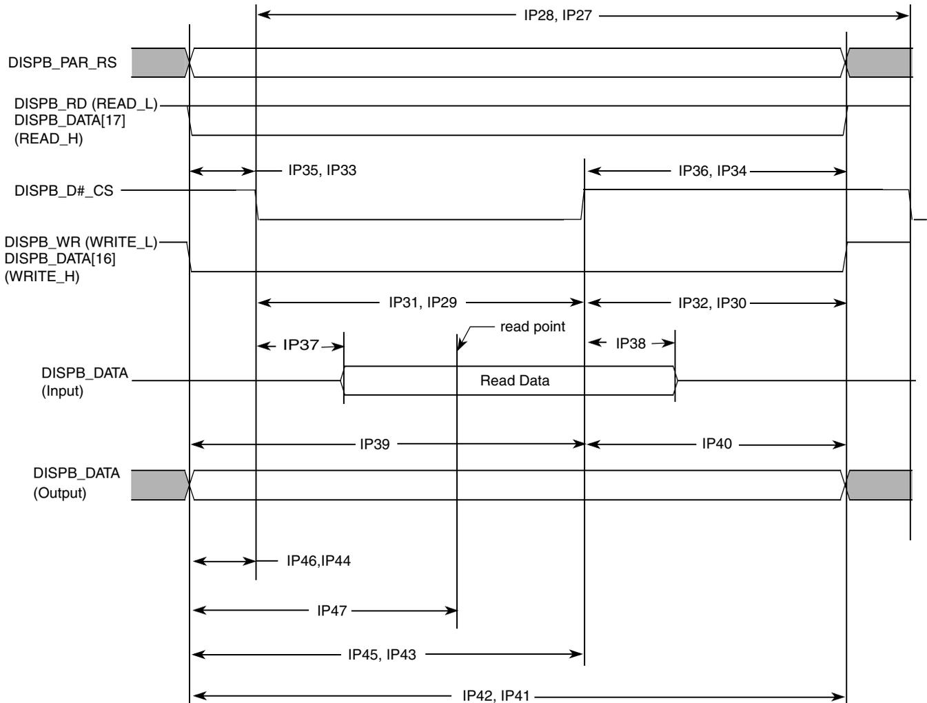
Figure 58. Asynchronous Parallel System 80 Interface (Type 1) Timing Diagram
