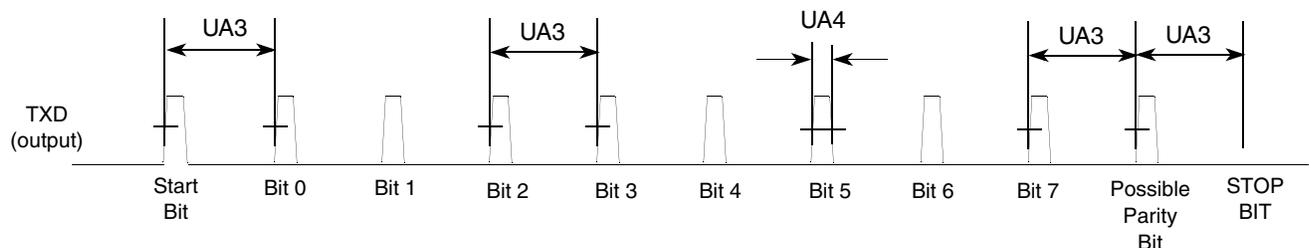
**Figure 98. UART IrDA Mode Transmit Timing Diagram**
