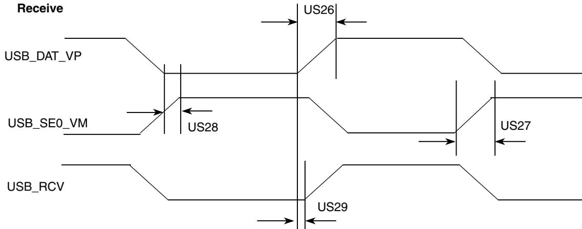
**Figure 105. USB Receive Waveform in VP\_VM Bidirectional Mode**
