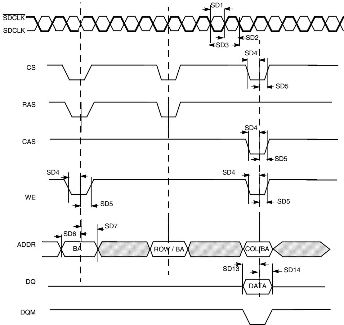
**Figure 28. SDR SDRAM Write Cycle Timing Diagram**
