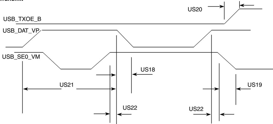
**Figure 104. USB Transmit Waveform in VP\_VM Bidirectional Mode**
