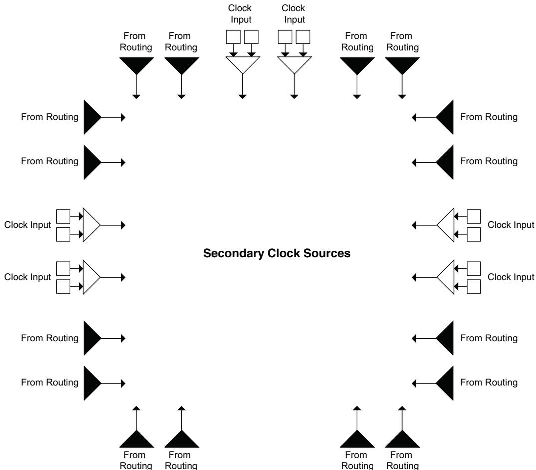
Note: Clock inputs can be configured in differential or single-ended mode.
