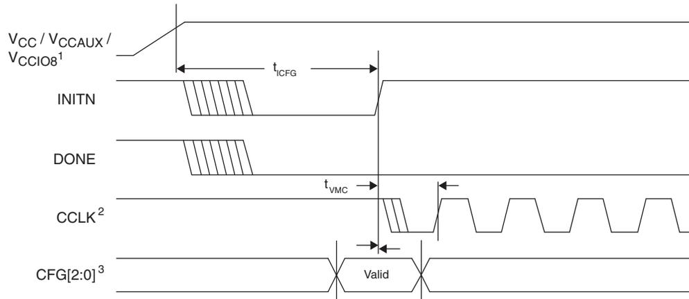
1. Time taken from  $V_{CC}$ ,  $V_{CCAUX}$  or  $V_{CCIO8}$ , whichever is the last to cross the POR trip point.
