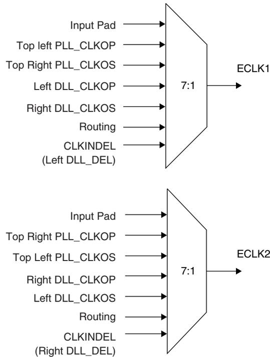
The edge clocks have low injection delay and low skew. They are used to clock the I/O registers and thus are ideal for creating I/O interfaces with a single clock signal and a wide data bus. They are also used for DDR Memory or Generic DDR interfaces.
