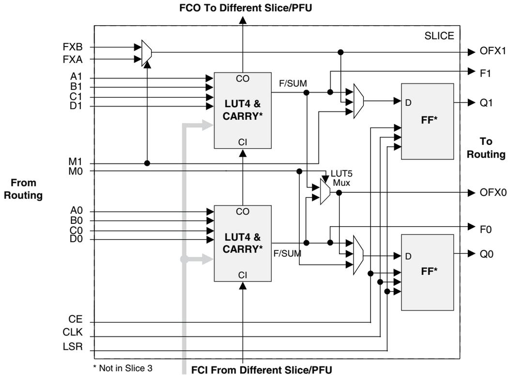
For Slices 0 and 1, memory control signals are generated from Slice 2 as follows:
