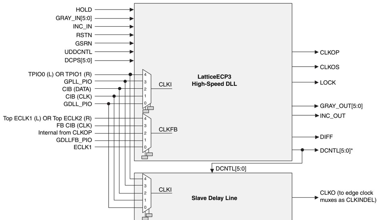
\* This signal is not user accessible. It can only be used to feed the slave delay line.
