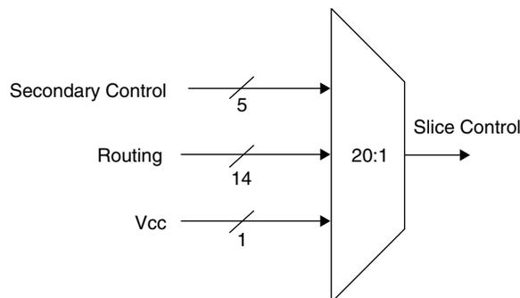
**Figure 2-25. Detailed sysDSP Slice Diagram**
