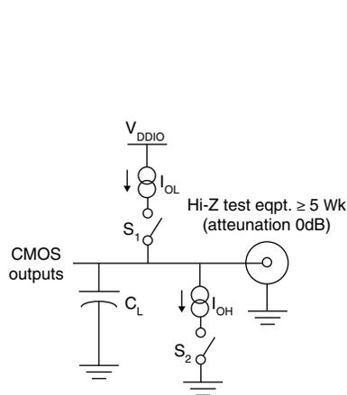
$C_L$  including probe and jig capacitance, 3 pF max.
