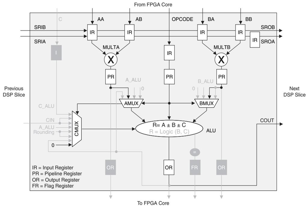
Figure 2-33. Input Register Block for Left, Right and Top Edges
