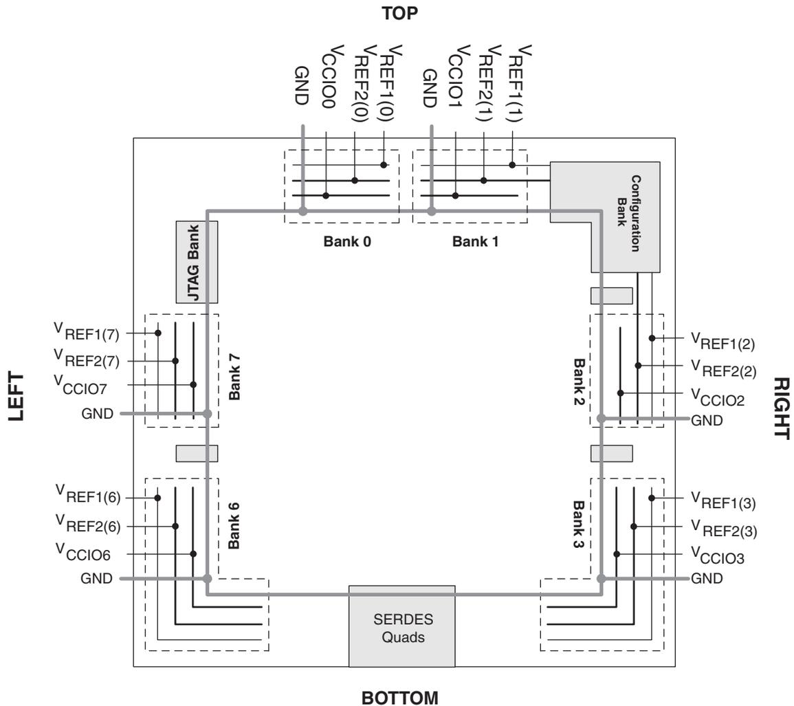
LatticeECP3 devices contain two types of sysI/O buffer pairs.
