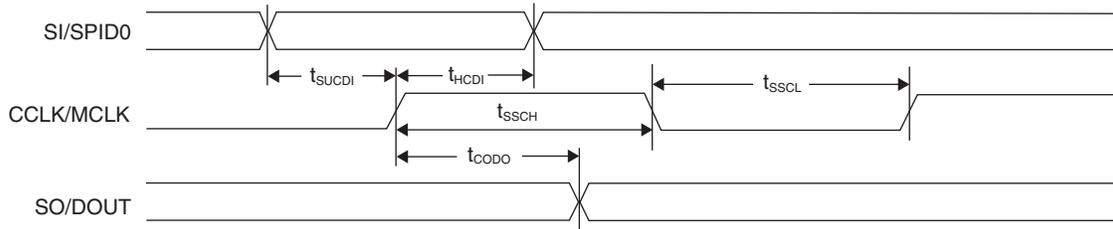
**Figure 3-31. Slave SPI HOLDN Waveforms**
