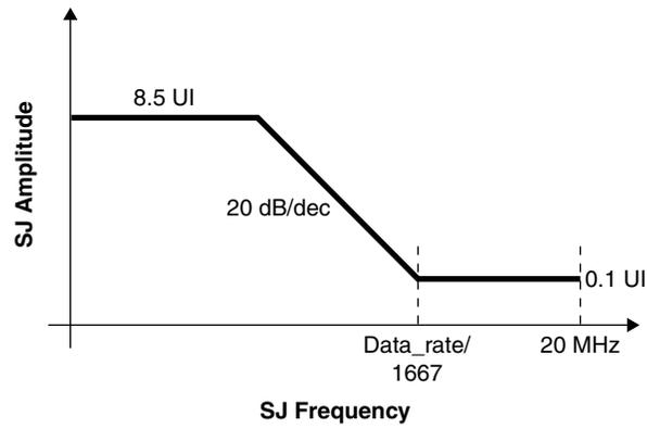
Note: The sinusoidal jitter tolerance is measured with at least 0.37 UIpp of Deterministic jitter (Dj) and the sum of Dj and Rj (random jitter) is at least 0.55 UIpp. Therefore, the sum of Dj, Rj and Sj (sinusoidal jitter) is at least 0.65 UIpp (Dj = 0.37, Rj = 0.18, Sj = 0.1).
