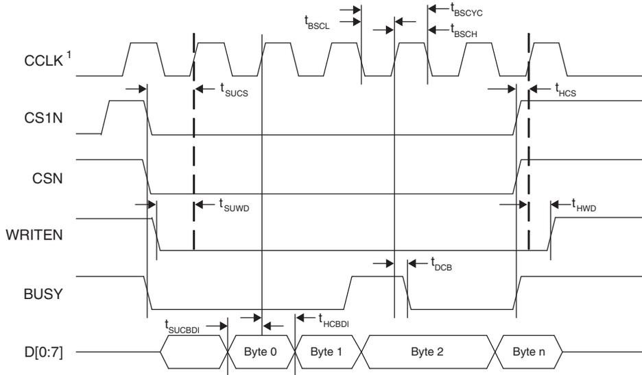
1. In Master Parallel Mode the FPGA provides CCLK (MCLK). In Slave Parallel Mode the external device provides CCLK.
