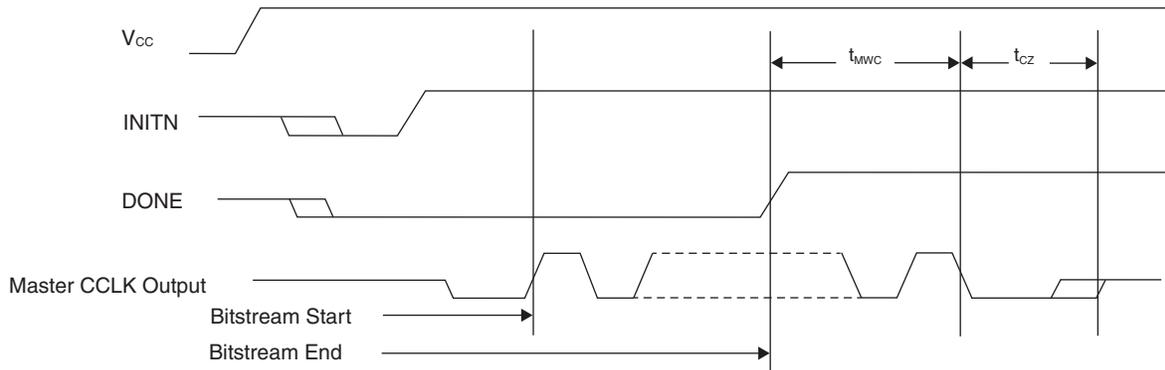
**Figure 3-28. Master SPI Configuration Waveforms**
