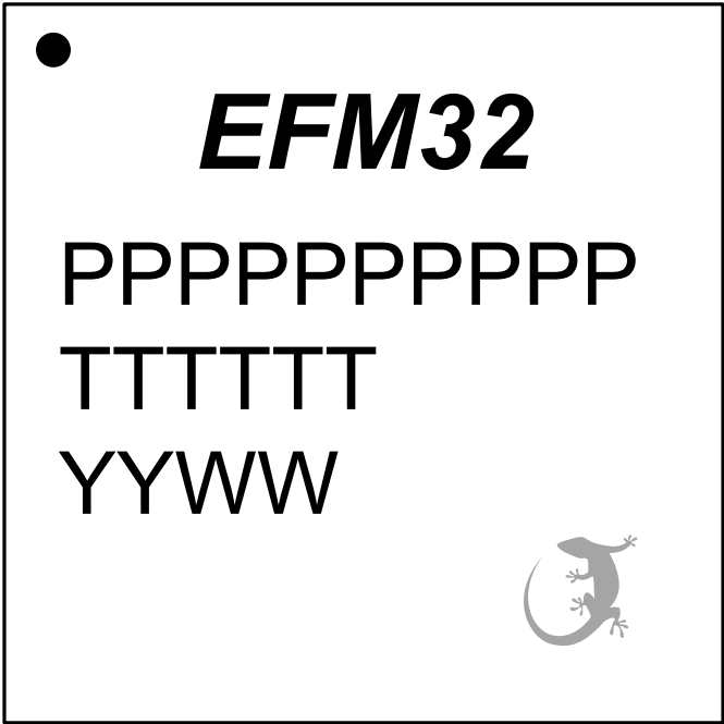
Figure 10.3. TQFP100 Package Marking
