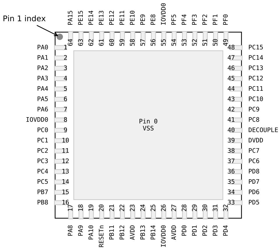
Figure 5.19. EFM32GG11B1xx in QFN64 Device Pinout
