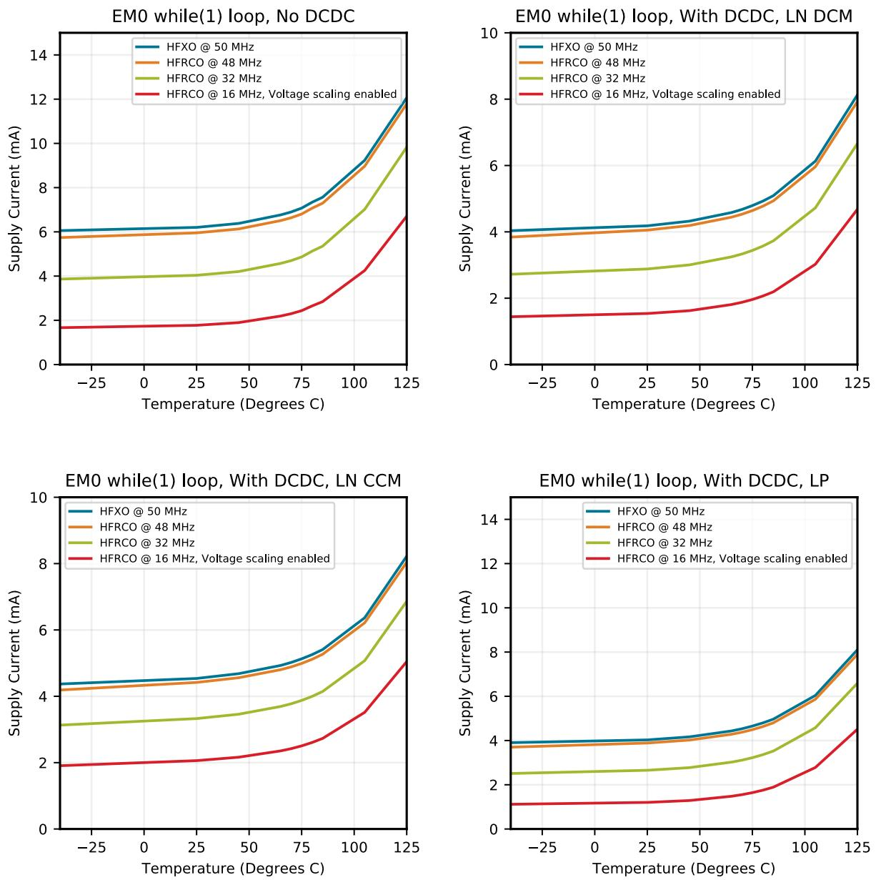
**Figure 4.24. EM0 Active Mode Typical Supply Current vs. Temperature**
