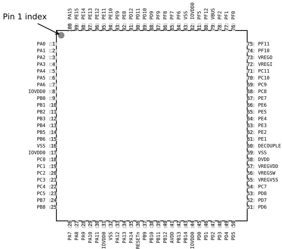
**Figure 5.8. EFM32GG11B8xx in QFP100 Device Pinout**
