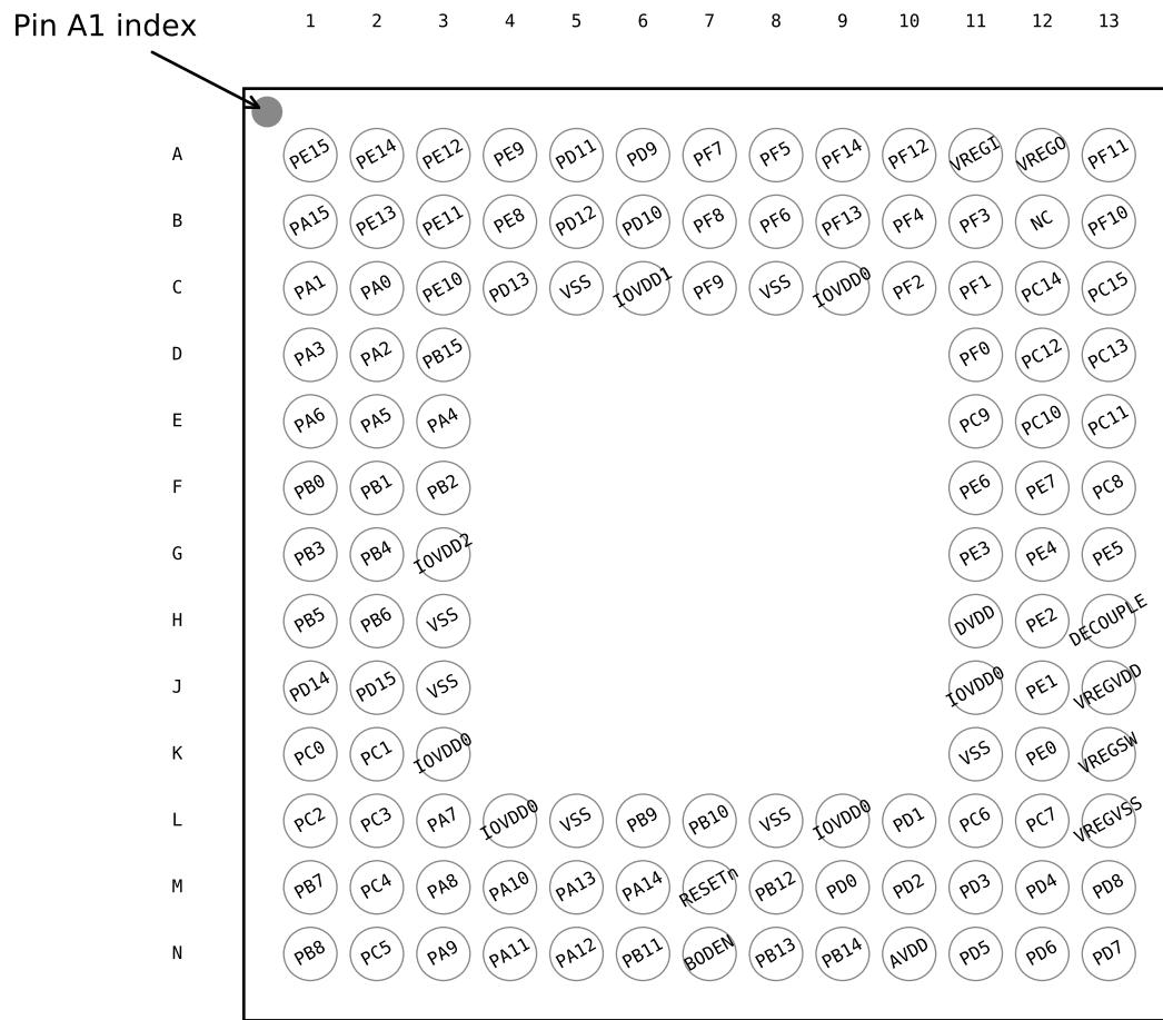
Figure 5.4. EFM32GG11B5xx in BGA120 Device Pinout
