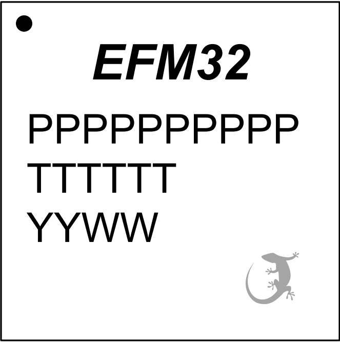
Figure 10.3. TQFP100 Package Marking
