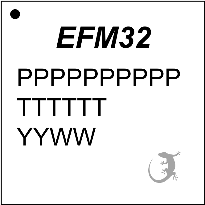
Figure 10.3. TQFP100 Package Marking
