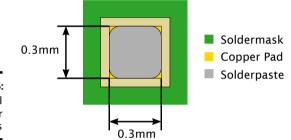
Figure 16: Solder stencil for outer pads
